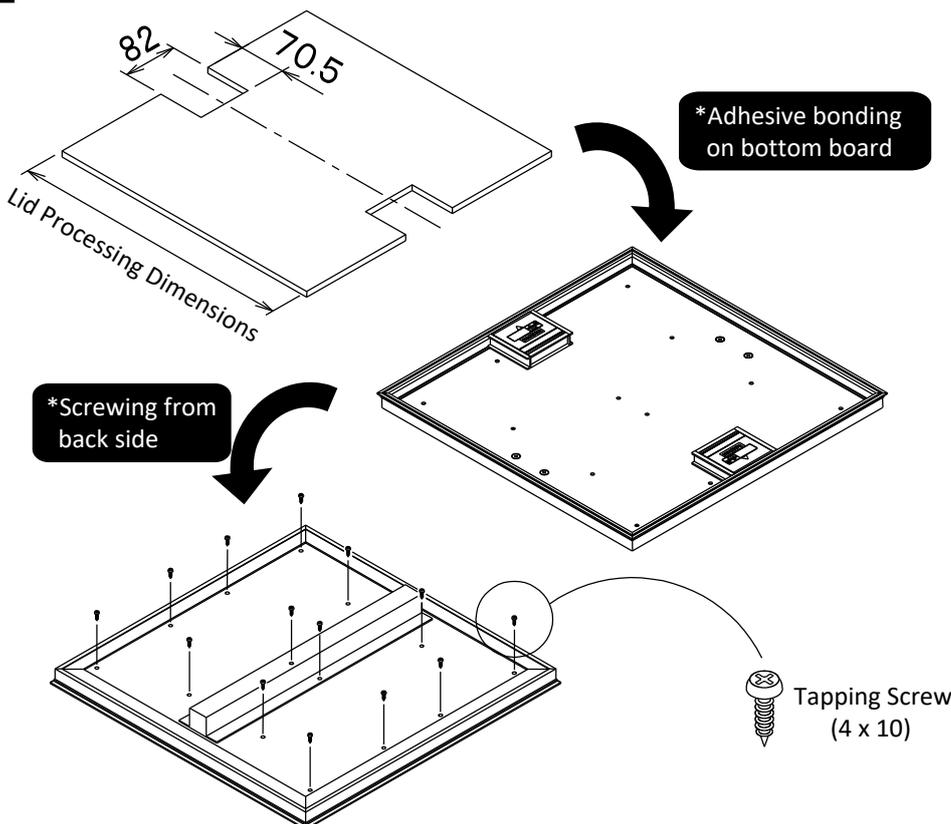
1. Cut the base materials according to the lid dimension and handle part (82 x 70.5) for each central part.
