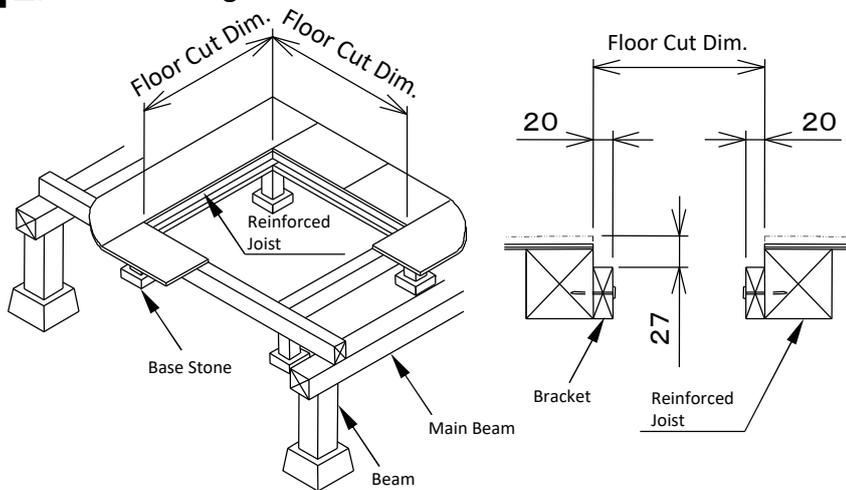
1. Cut the floor opening according to the floor cut dimension, and then attach the reinforced joint all around beneath the floor.
