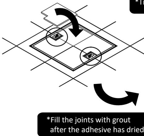
1. Cut the tile according to the outer frame and inner lid.
