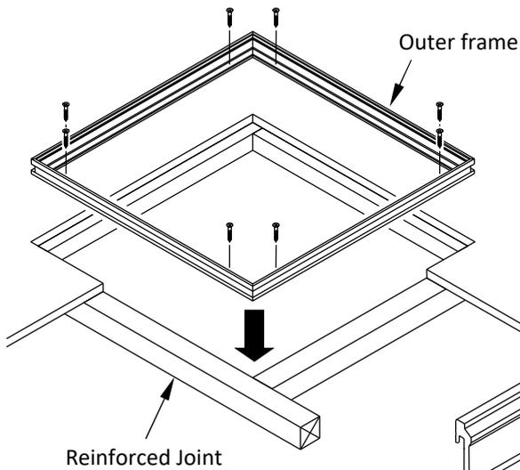
1. Mount the outer frame in floor cut space
