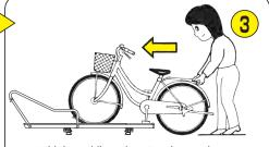
Hold the saddle and carrier, then push forward. Make sure to confirm that the front and rear wheels are stored properly.
