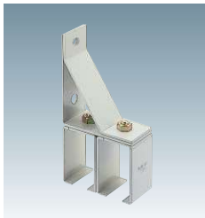
Wall Bracket (Double Track) #4 SB2 •Assembly bolt of box and Stay are all W1/2" countersunk bolt. •Recommended mounting Screw: M12
