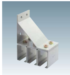
Rail Joint Bracket for Wall (Triple Track) #4 SBT3 •Assembly bolt of box and Stay are all W1/2" countersunk bolt. •Recommended mounting Screw: M12
